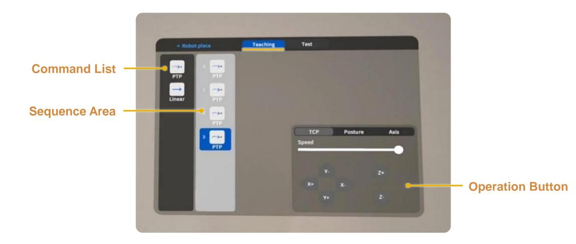
**Teaching** Operate the robot and create a operation program for its movements.
