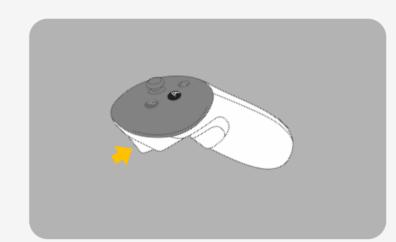
Press the trigger button on the right controller briefly to reset the position and size of the operation panel, placing it in front of the operator.
