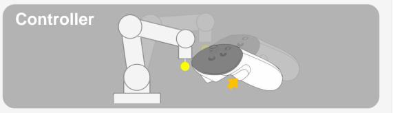
Hold the controller close to the object and move it while holding down the grip button.
